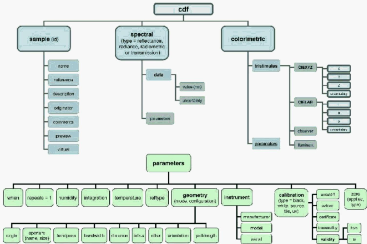
Figure 2 — Parameters that can be associated with each measurement block
